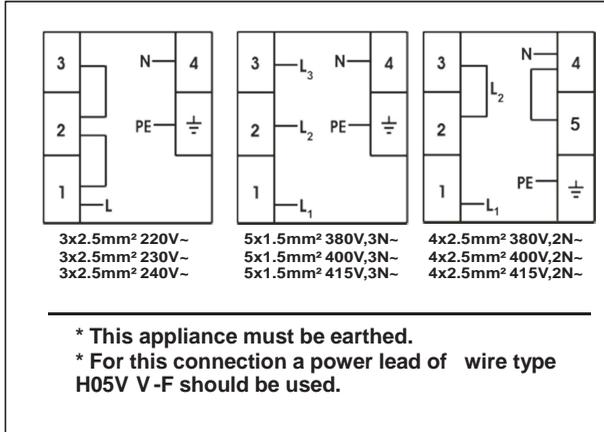
For the induction hob, the cable must be H05VV-F 3X2,5 mm<sup>2</sup>/60227 IEC 53 ••. You will find the connection diagram shown on the bottom of your appliance.
