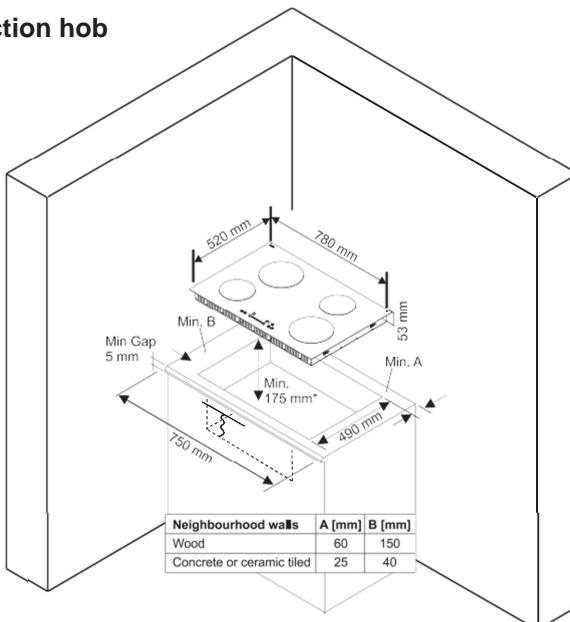
\* : In the case of installation over built in oven, distance should be min. 10 mm.
