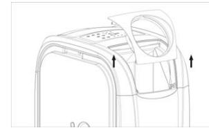
1. Remove the exhaust tube from its storage under the rear air outlet. Replace the rear air outlet.
