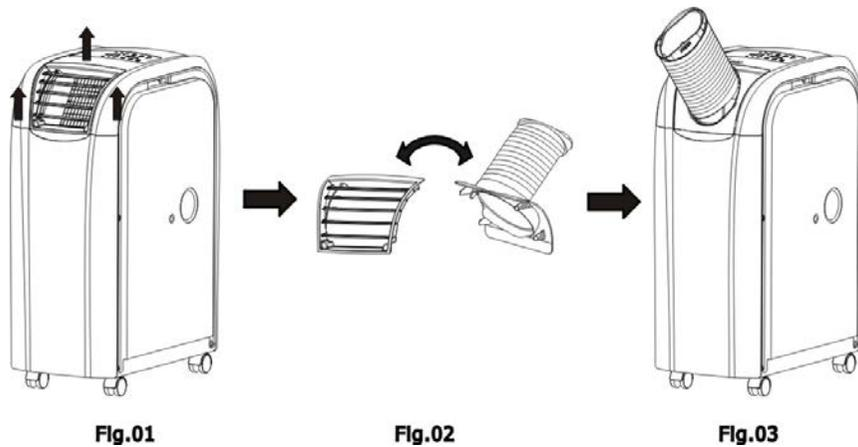
The outlet exhaust must still be attached to the window when using the heating function.
