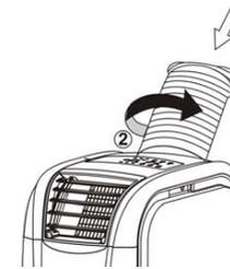
2. Install the exhaust tube by rotating it clockwise onto the rear air outlet. Please ensure it is fully inserted before use.
