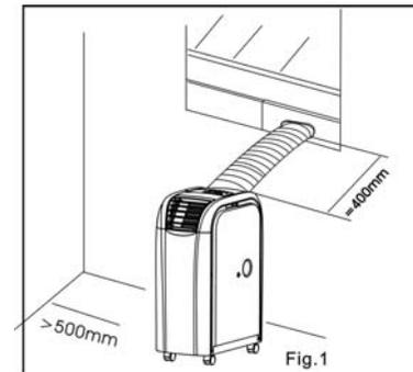
Install the portable air conditioner in a flat location with adequate space to ensure the air inlets and outlets will not be blocked.
