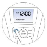
Step-2: Simply pressing Hour and Min keys to select brewing time. The scheduled time will display on LCD.
