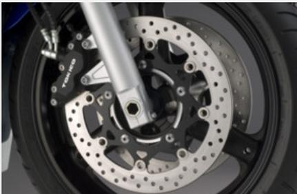
Dual front disc brakes use four-piston Tokico calipers, with two pistons on each side of the caliper, and 310mm floating discs. The rear brake combines a Nissin caliper with a 240mm.
