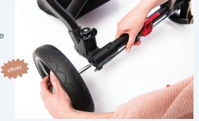
Next, insert each front wheel pin into the centre of the socket ensuring you hear them "click" in. Give each wheel a firm tug to ensure they are secure.
