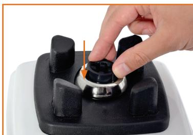
2. Remove existing rubber drive gear using small pliers, gently pull up to pull the gear out.
