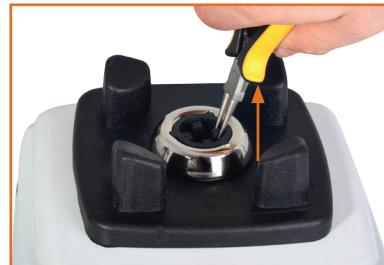
1. Ensure motor is unplugged from outlet and that you have the spare rubber drive gear ready.
