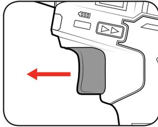
**Note:** The more the variable speed trigger is depressed, the faster the drill bit will rotate.
