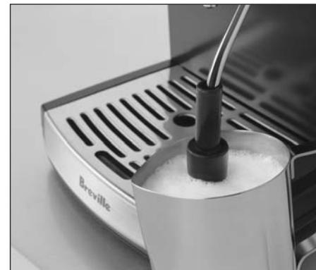
If steam starts coming from the Steam Wand before it is immersed in the milk, pause the steam by turning the Selector Control back to the 'STAND BY' position. This will avoid the steam pressure blowing milk out of the jug. A pumping noise will sound for a short time.
