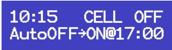
The first line of the display shows the current time and the cell status and output. In the example above the time is 10.15am and the Cell is "OFF". If the Cell is on, the output of the Cell will be displayed. If the output of the Cell has been set at lower than 100%, "CELL OFF" will be displayed intermittently even while the unit is running as the Cell regulates output. (See Chlorine Output Menu on page 16 for more details)
