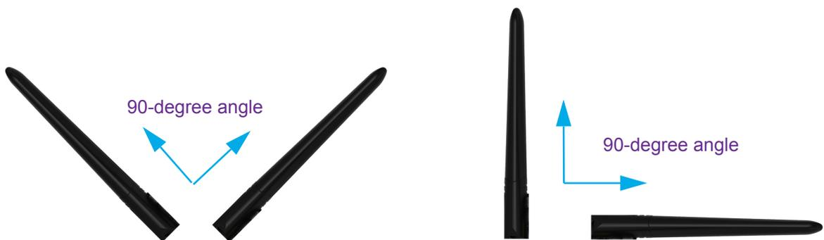
Figure 4. Recommended antenna angle
